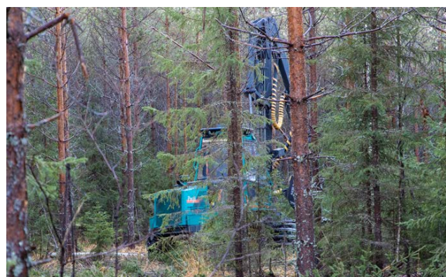
Harvester in a thinning operation
