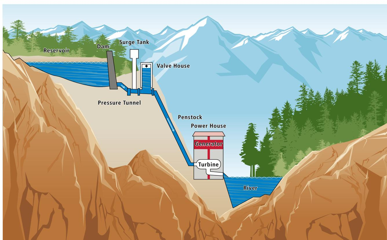
It is also important to take into account the flexibility required regarding the various rates of flow in a typical run-of-river plant. A Pelton turbine is highly flexible over a range of water flows. Therefore, if there is a highly variable water flow throughout the year, it would often be best to use a Pelton turbine.
